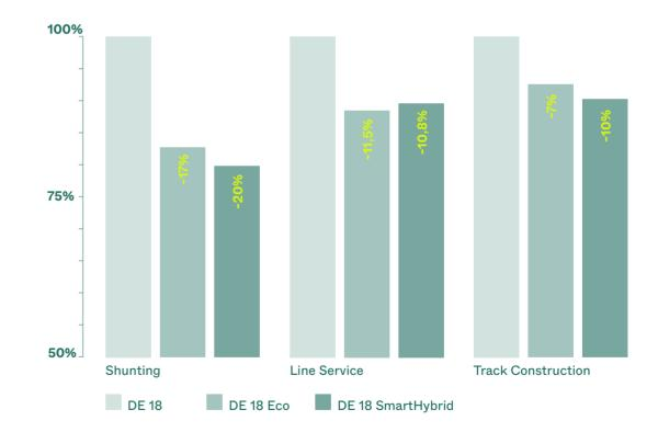
Simulation data is provided by real operational scenarios. Rated engine power is reduced to 1200 kW in ECO-mode. Rated engine power is reduced to 1500 kW in Smart Hybrid mode.
